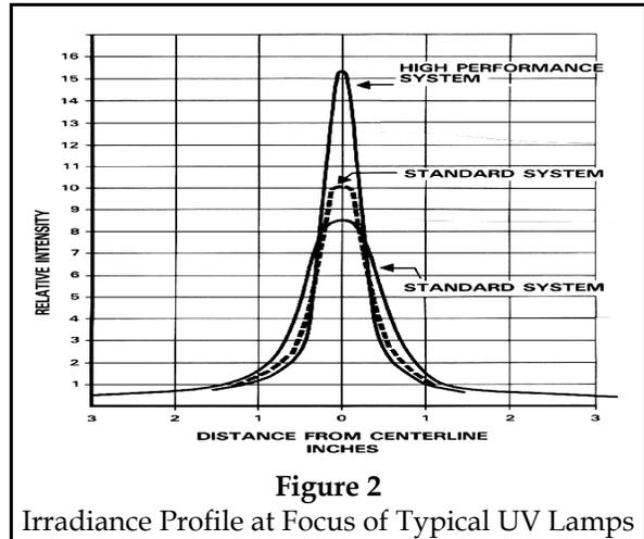
The elliptical reflector is generally the highest efficiency of reflector, as it has the greatest "wrap," or included angle of reflected energy about the bulb. Often reflector shapes other than the simple ellipse are considered. Table I shows the relative merits, measured by speed to achieve cure of a black screen ink. This demonstrates the effects of bulb diameter and reflector geometry with lamps of the same power, but different peak irradiance and optical efficiency.<sup>(5)</sup>
